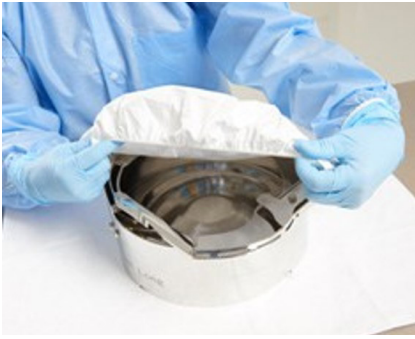
Figure 1: To apply a Purefit elasticized cover, stretch it over the opening, then pull the sides downward
