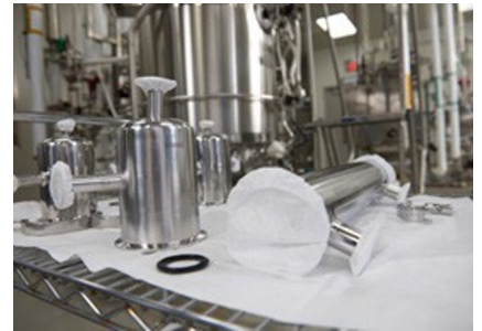
Figure 2: Properly sized and applied Purefit elasticized covers achieve a close fit optimized for steam sterilization
