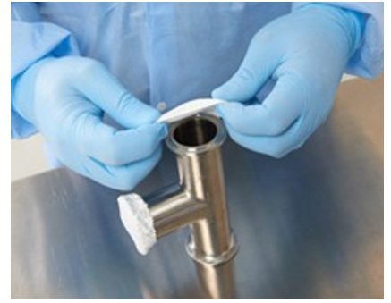
Figure 1: To apply a Purefit elasticized cover, stretch it over the opening, then pull the sides downward
