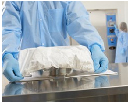
Figure 1: To apply a Purefit elasticized cover, stretch it over the opening, then pull the sides downward
